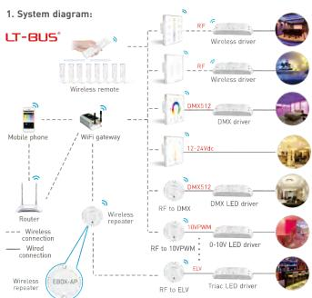
EBOX-AP wireless repeater applies LT-BUS wireless communication protocol for wireless signal extension, it is not necessary to pair via its factory default setting, greatly ensures its stability and wide controlling area among LT-BUS wireless communication devices, removing the complex cabling procedure, to make it become more easier for new or retrofit installations.
